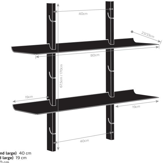
Distance between holes (both small and large) 40 cm Outside shelf distance (both small and large) 19 cm Shelf length (both small and large) 80 cm Wall to shelf edge (short 23 cm) / (large 33 cm) Height of rails (short 67,5 cm) / (large 170 cm)
